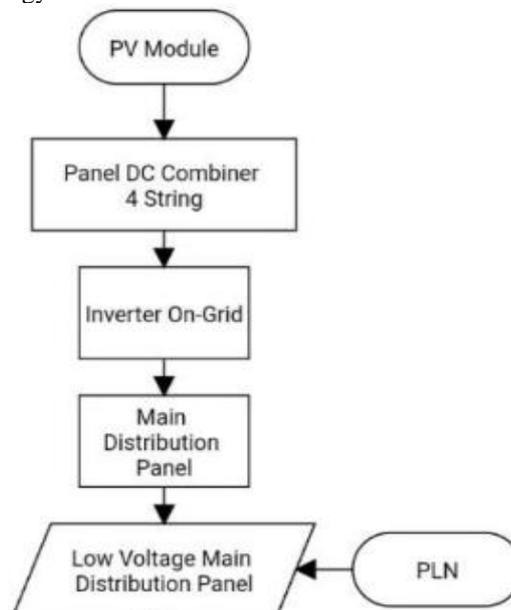
Figure 1. Block diagram of rooftop solar power plant
