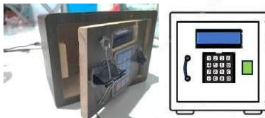
Figure 5. Tool Design in Open and Closed Conditions
