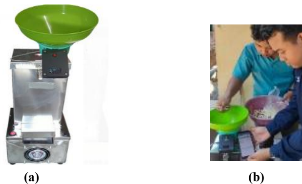
Figure 8. (a) Modified peeling machine; (b) field testing of the system at onion processing SMEs
