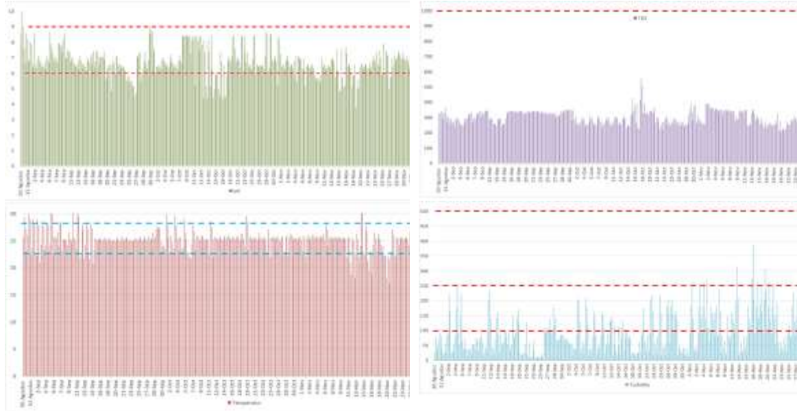
Figure 5. Graph of pH, Temperature, TDS and turbidity parameter values during the monitoring period (morning, afternoon, evening, night)
