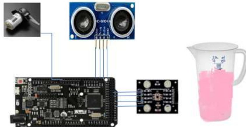
Figure 2. Titration Control System Design
