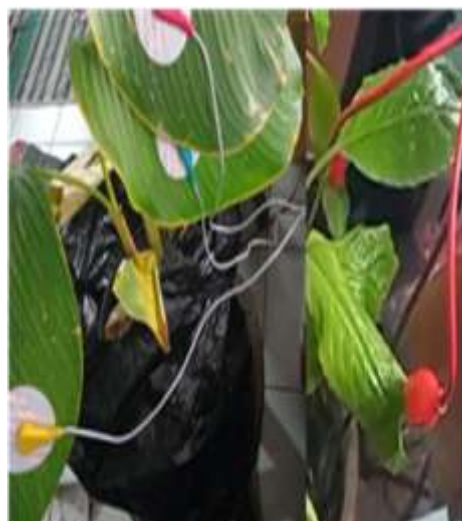
Figure 7. Electrode placement on the plant
