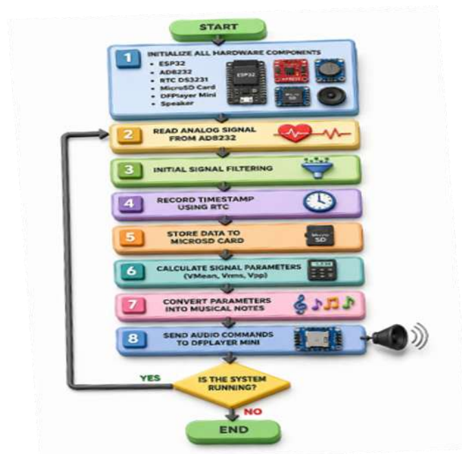
Figure 5. Implementation of the bioelectrical sensor using the AD8232 module
