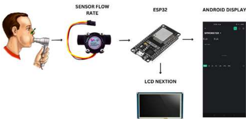
Figure. 1. The Diagram Block of Real-Time Lung Function Measurement with Flow Meter and Android Display
