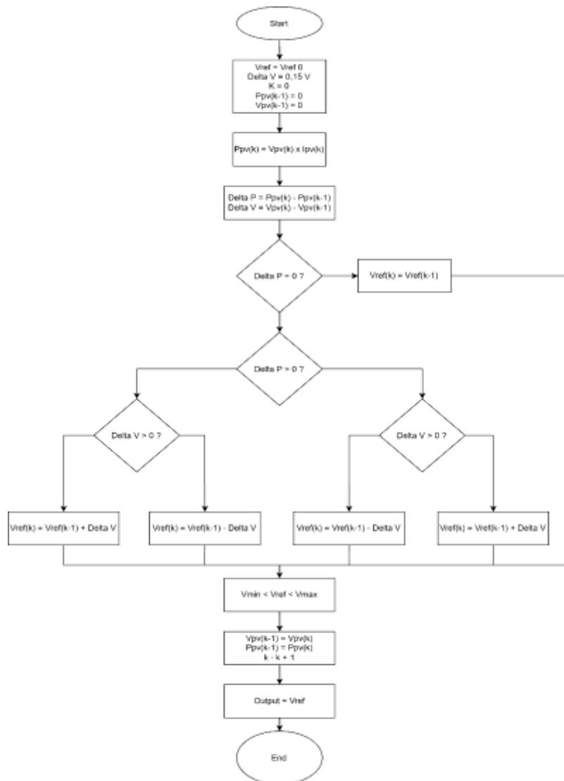
Figure 4. MPPT Perturb and Observe Flowchart.
