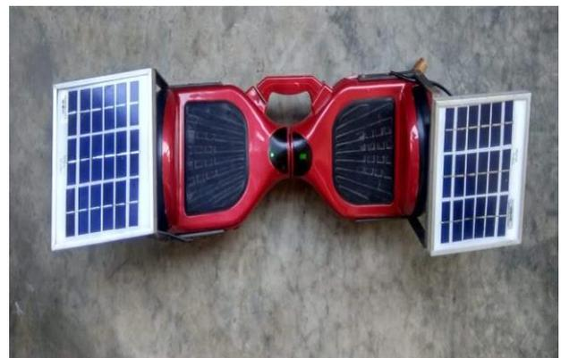
Fig. 12 final shape of the multi way charging hover board
