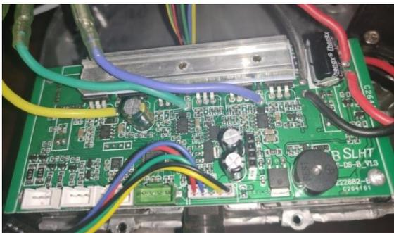
Fig. 3 Master control board
