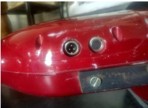
Fig. 11 Charging port and Pressure switch
