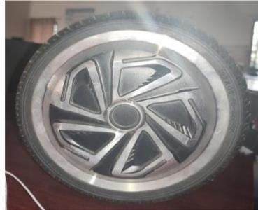
Fig. 8 BLDC hub motor
