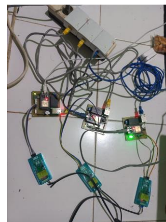
Gambar 11. Hardware Pengujian Kounikasi Sistem 3 Slave 1 Master
