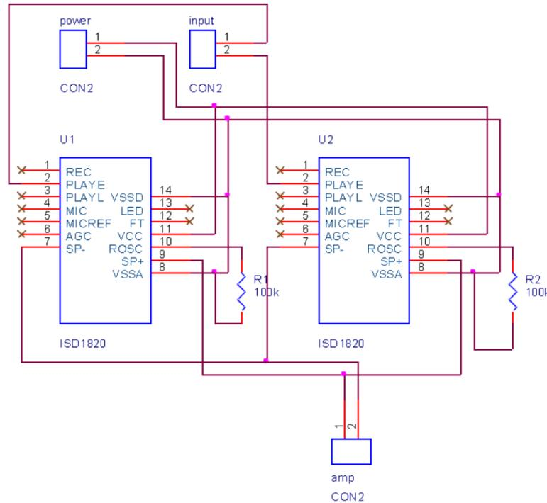
Figure 3. ISD 1820 wiring module system
