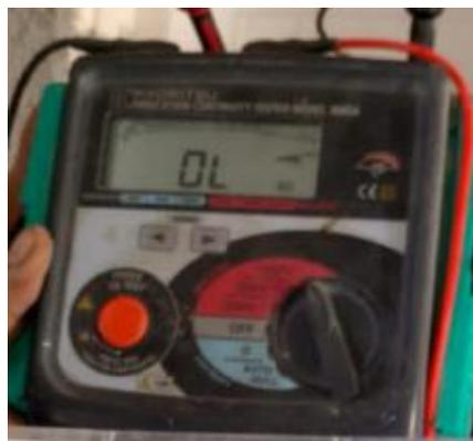
Gambar 2. *Insulation Continuity Tester*
