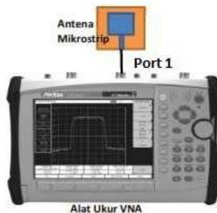
Figure 2. Antenna Measurement Configuration Using VNA
